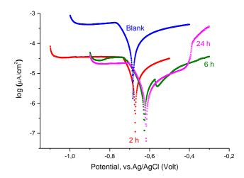
FIGURE 2. Potentiodynamic current potential curves of aluminum in  $0.5 \text{ M H}_2\text{SO}_4$  in the presence of *Cannabis sativa* L. extract with during 2 h, 6 h and 24 h.
