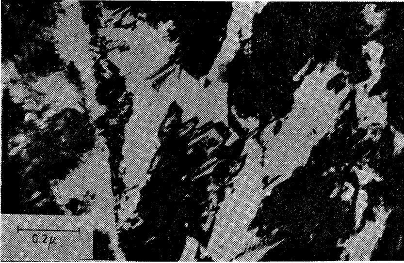
FIGURE 3. Electron micrograph of austenite-martensite region. Dark area shows the massive martensites in which mechanical twins formed.
