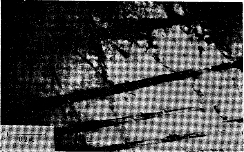
FIGURE 1. Transmission electron micrograph of Ti-62 % Ta alloy showing dislocations. Thicker dark bands show plate martensites.
