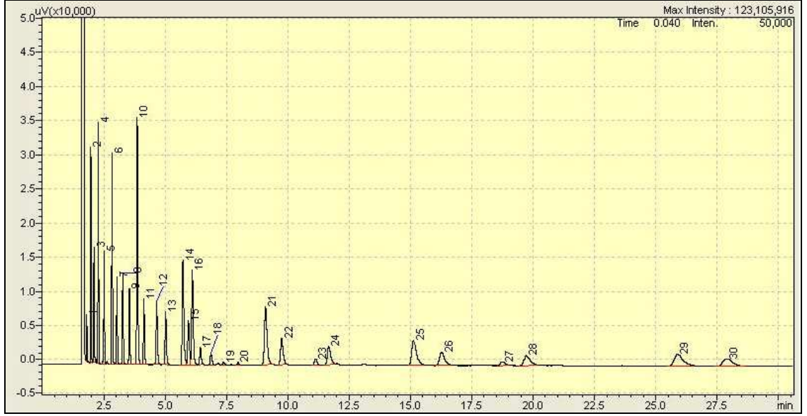
Şekil 3.1 Yağ asitleri standartlarına ait GC kromatogramı (1; miristik ( C14:00), 2; palmitik asit (C16:00), 3; palmitoleik asit (C16:01), 4; margarik asit (C17:00), 5; margaoleik asit (C17:01), 6; stearik asit (C18:00), 7; oleik asit (C18:01), 8; linoleik asit (C18:02), 9; linolenik asit (C18:03), 10; eikosaik asit (C20:00), 11; cis 11 eikosaik asit (C20:01), 12; eikosadionaik asit (C22:00))
