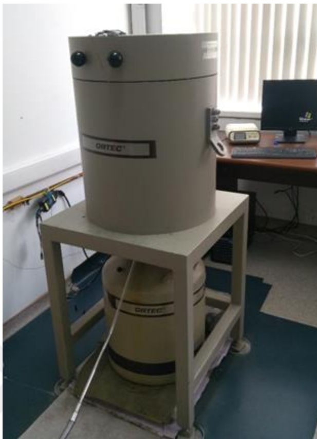
Figure 3.12 A photograph of the HpGe Detector used in experiments
