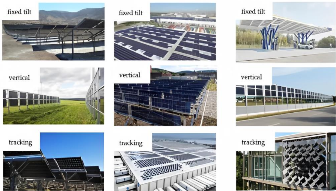
Figure 2.2 Various bifacial PV systems installation configurations and applications (Kopecek, 2021)
